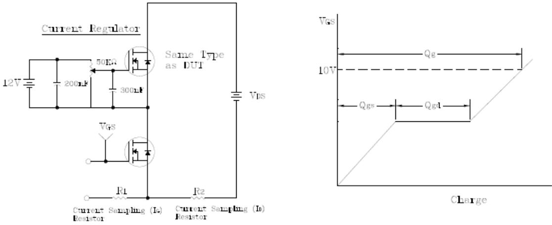
**Fig. 13 Resistive Switching Test Circuit & Waveform**
