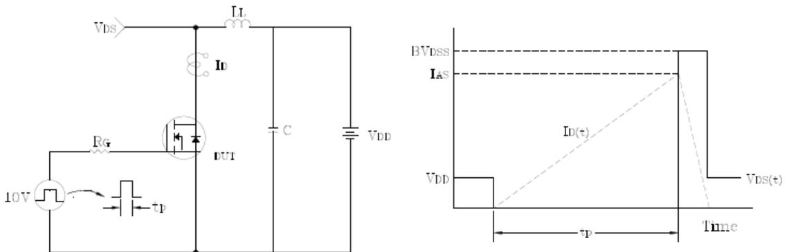
Fig. 15 Diode Reverse Recovery Time Test Circuit & Waveform
