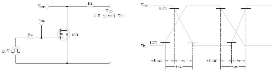
**Fig. 14 EAS Test Circuit & Waveform**
